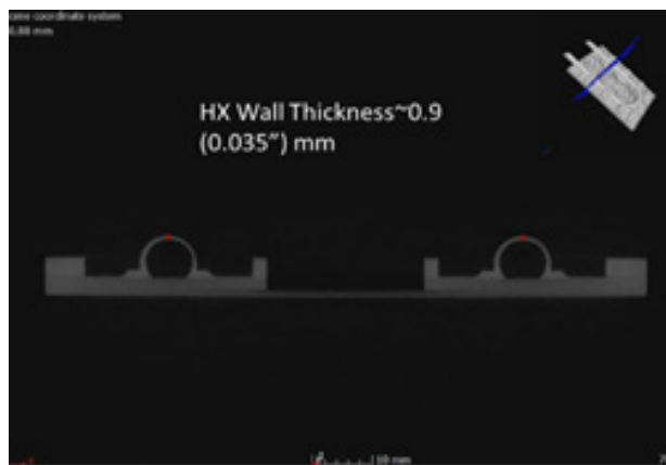
Figure 4 - Stringent ground-based space-grade qualification testing of UAM heat exchanger devices. EWI helped Fabrisonic complete CT Scanning and helium leak testing of UAM heat exchangers throughout development.
