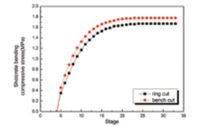
Comparison of bending compressive stresses in shotcrete between different excavation methods
