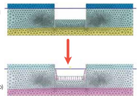
Automatic application of water pressure on excavated face below the water level
