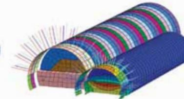
Comparison of results between different excavation methods in the same model file
