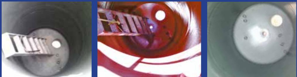
*(Left) Re-inserting newly coated coil into lined reactor. (Right) Completed unit with mixer, coil and reactor ready for hazardous acid service once again.*
