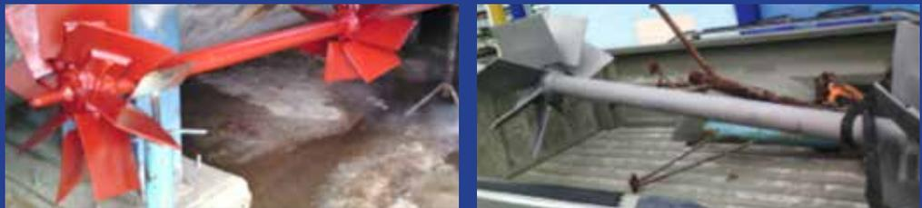
*(Left) After blasting, now preparing to line the reactor. (Center) First coat of ChemLine® applied. (Right) Top coat of ChemLine® applied and heat cured.*
