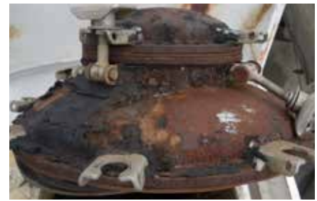
(Photo 1) Interior pitted tank with corrosion prior to ChemLine® application. (Photo 2) Finished tank with ChemLine® coating.
