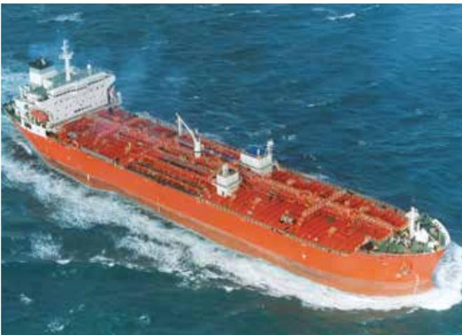
**Marine tanker with MarineLine cargo tanks.**
