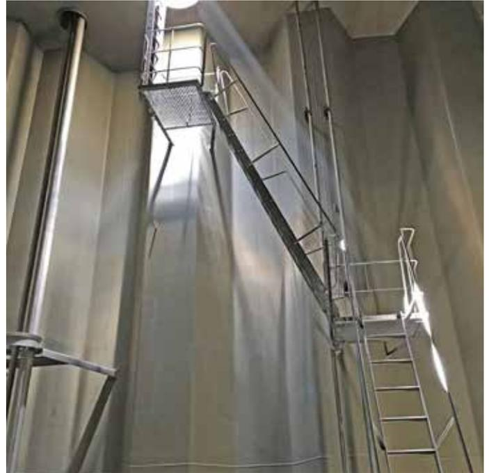
**After a recent onboard inspection, the eight-year old MarineLine® cargo tank coating on the *M/T Borchali* is shown in excellent condition.**
