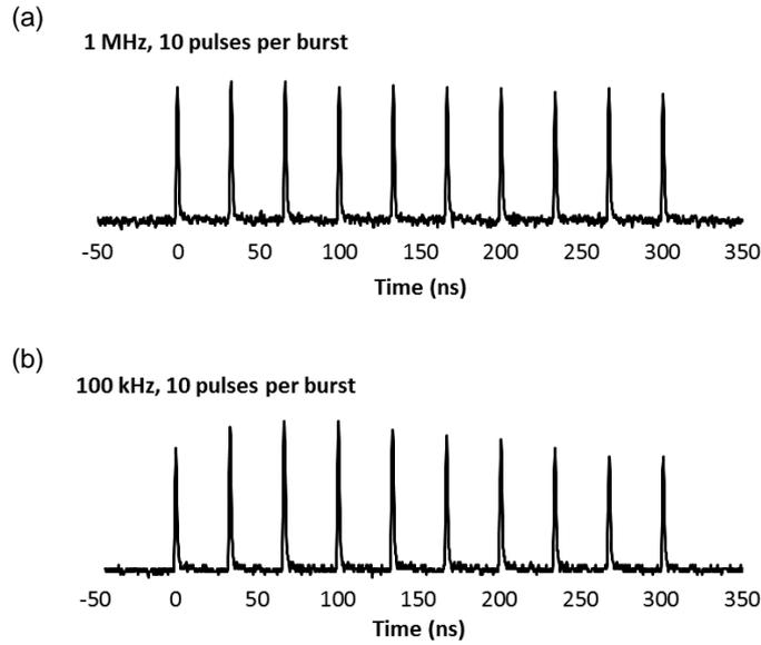
Figure 6. Amplified burst pulse traces with 10 pulses per burst at (a) 1 MHz and (b) 100 kHz repetition rate.
