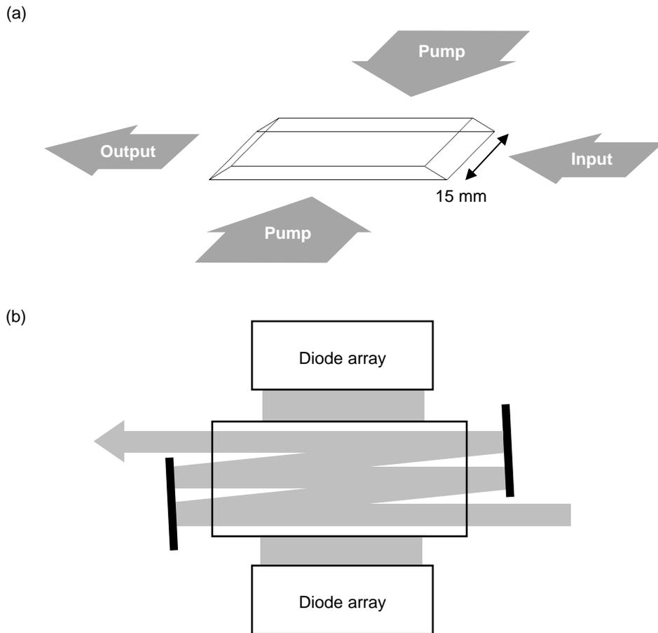
Figure 1. Schematic of Z-slab showing (a) slab shape and (b) multi-pass configuration.
