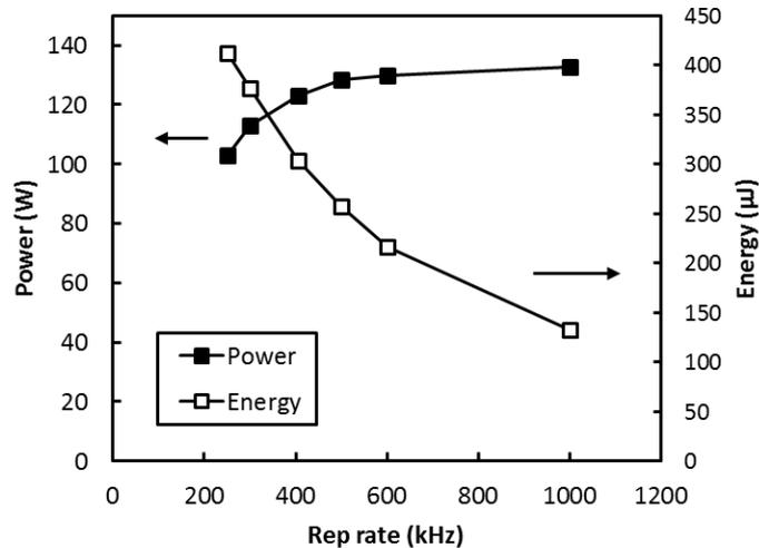
Figure 4. Average power and pulse energy as functions of repetition rate.
