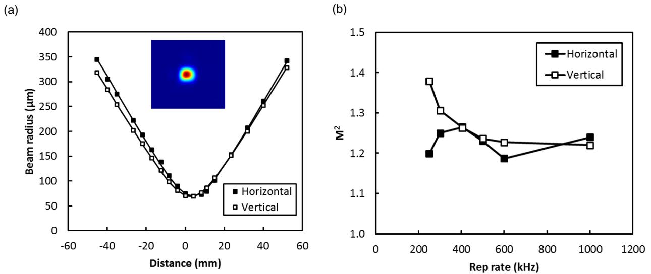
Figure 5. (a) Horizontal and vertical caustics at maximum power and 400 kHz repetition rate ( $M_x^2, M_y^2 < 1.30$ ) with beam profile at the waist position (inset) and (b)  $M^2$  vs repetition rate at full pump power.
