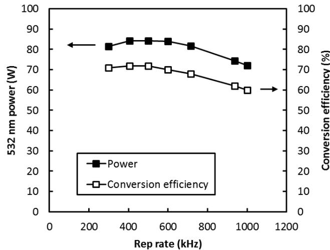
Figure 8. Power at 532 nm and conversion efficiency as a function of repetition rate for laser system with SHG module.
