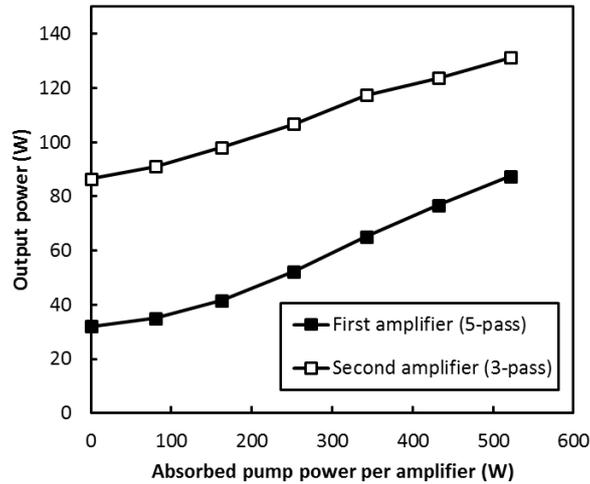
Figure 3. Power curves for both Z-slab power amplifiers at 400 kHz repetition rate.
