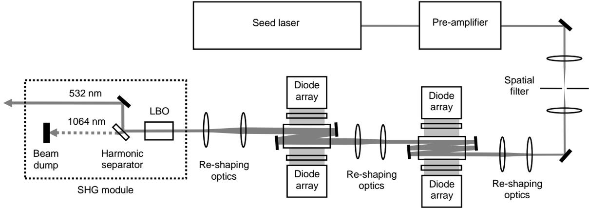
Figure 2. Schematic diagram of MOPA system with second harmonic generation.
