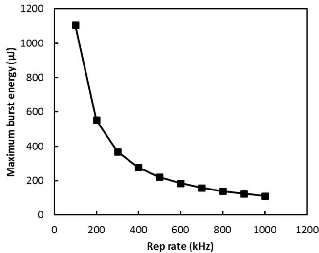
Figure 7. Maximum total burst energy as a function of repetition rate.
