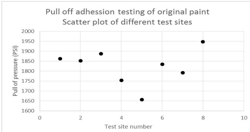
Figure 9. Distribution of pull off adhesion test measurements over 8 sites of painted samples prior to any laser depainting.
