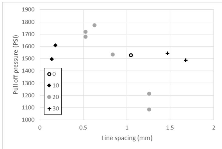
Figure 11. Pull off adhesion test results grouped by defocus and plotted against line spacing.
