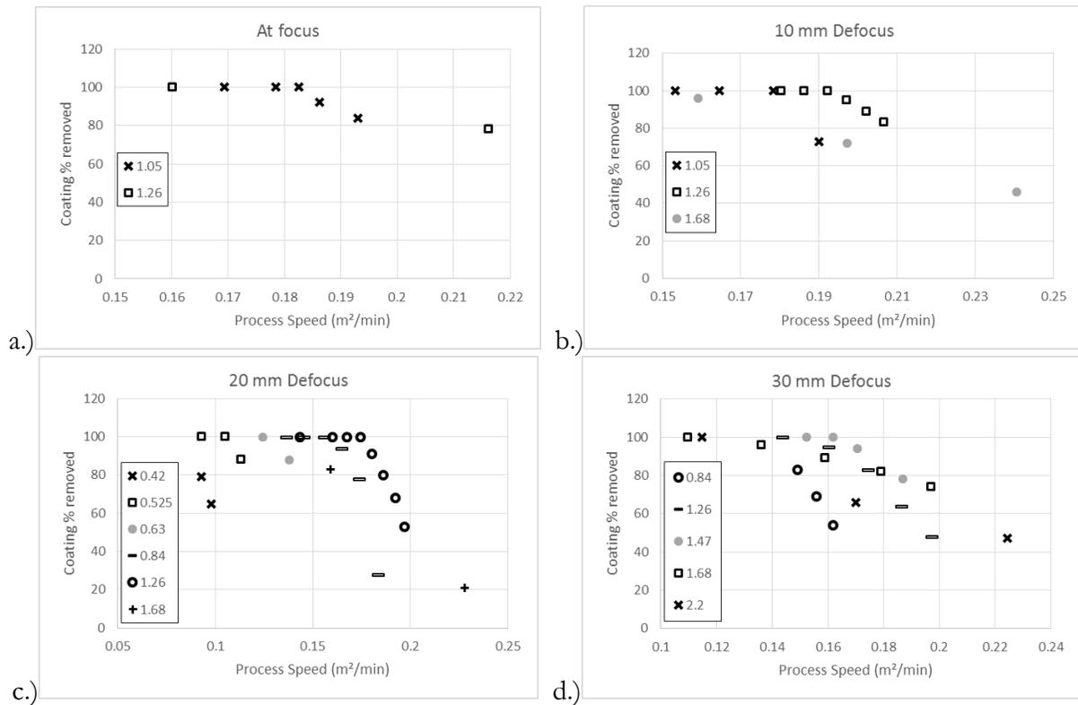
Figure 8. Coating percentage removed in different process speeds, results grouped by line to line spacing. a) Processing at focus, b) processing at 10 mm defocus, c) processing at 20 mm defocus, d) processing at 30 mm defocus.
