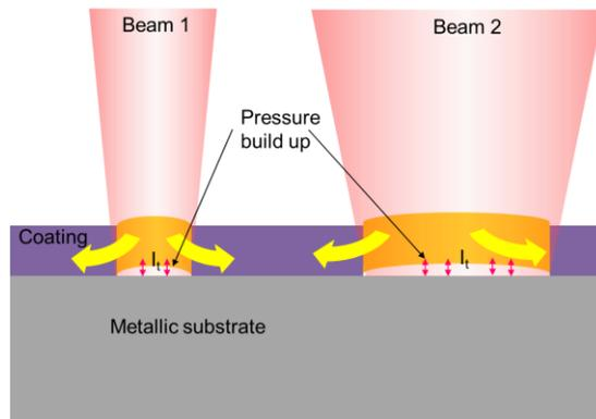
Figure 3: Sketch of detachment comparing large and small beams
