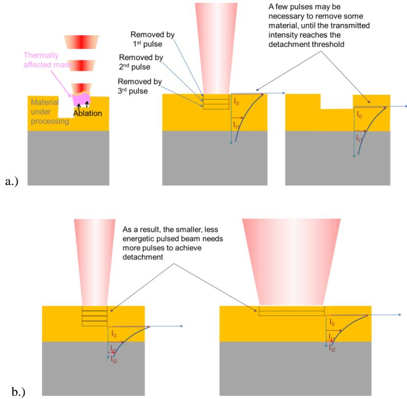
Figure 4: Sketch of hybrid detachment phenomenon. a.) Mechanism of hybrid detachment b.) comparison of high and low pulse energy
