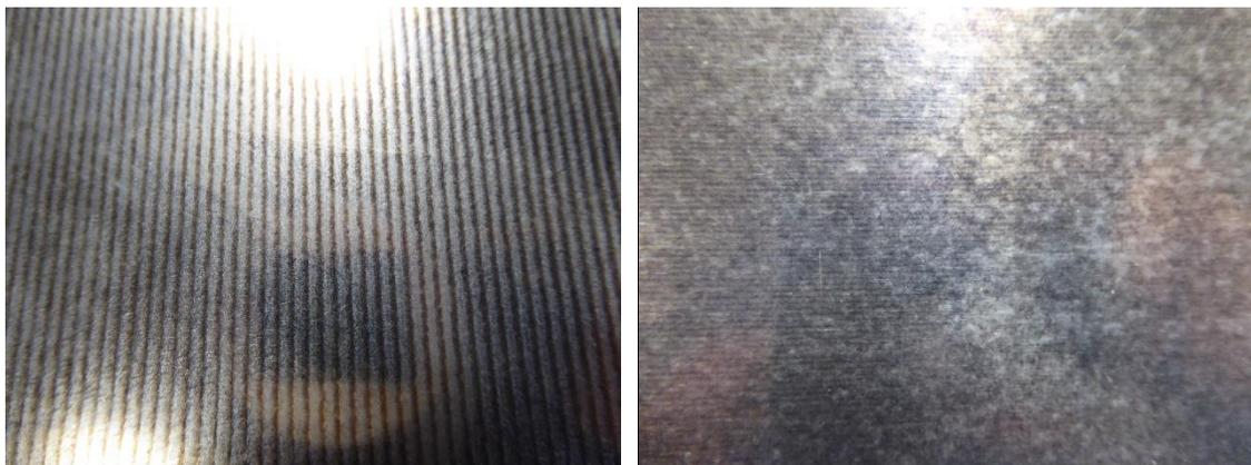
Figure 12. Left) laser depainted site with line spacing of 1.26 mm, 100 % coating removal. The darker lines are remaining chromate. Right) Laser depainted site with line spacing of 0.53mm, 100 % coating removal.
