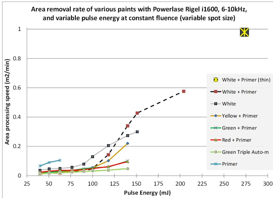
Figure 5: Removal rate data for various types and thicknesses of paint and paint/primer combinations
