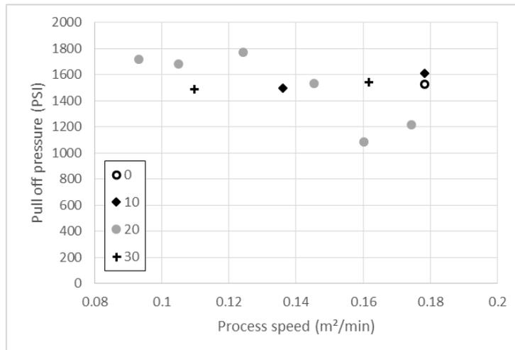
Figure 10. Pull off adhesion test results grouped by defocus and plotted against process speed.
