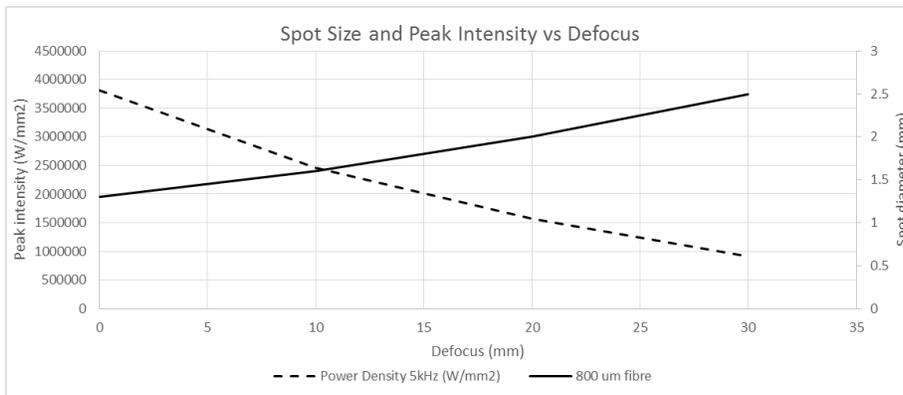
Figure 7. Variation of laser spot size diameter and pulse peak intensity, against distance from optimum focus of the f-theta scanning lens.
