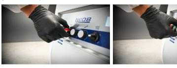
Pull out the blade speed, tumbler speed, and fan speed dials on the Variable Function display. Turn to the desired settings.
