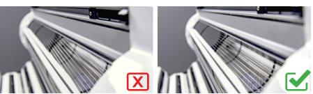
Pro Tip – try to straighten the tumbler cables as much as possible. When the tumbler is not straight it is shorter, making it difficult to lock the retaining ring on the outfeed side.
