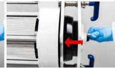
As air is pumped in, the Spring Compressor Tool will expand and push on the blue ring. Once the retaining ring is recessed inside the lid, the Spring Pack has been fully compressed and the retaining ring on the outfeed side can be installed.
