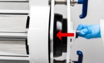
As air is pumped in, the Spring Compressor Tool will expand and push on the blue ring. Once the retaining ring is recessed inside the lid, the Spring Pack has been fully compressed and the retaining ring on the outfeed side can be removed.
