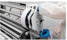
**The lid must be open to complete the following steps.** Lock the wheels, open the lid and insert the Spring Compressor Tool.
