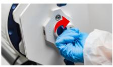
Turn the valve button to the closed position (pointing away from the Schrader valve).
