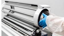
On the infeed side of the lid, remove the blue retaining ring by rotating to the unlock position, then pull the tumbler through the infeed side.
