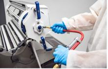
Apply compressed air into the Schrader valve. A hand pump will also work but with compressed air, this will only take a few seconds. **CAUTION: inflate to MAX 90 psi.**
