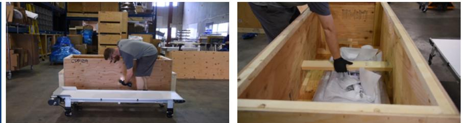
Unscrew the single 2x4 in the centre from the outside securing the legs.
