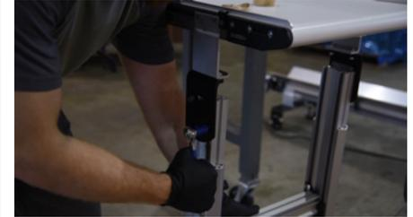
Follow the same process to install the legs on the opposite side, and on the infeed conveyor.
