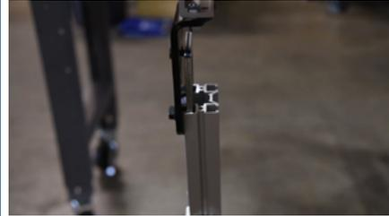
The wider, shorter set of legs are for the outfeed conveyor. Line up the legs on the inside of the black bracket so the u-bracket slides into the hollow groove on the outside of the legs.
