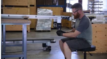
Set the conveyor on a table to allow the black brackets to dangle. Remove the rubber bands.
