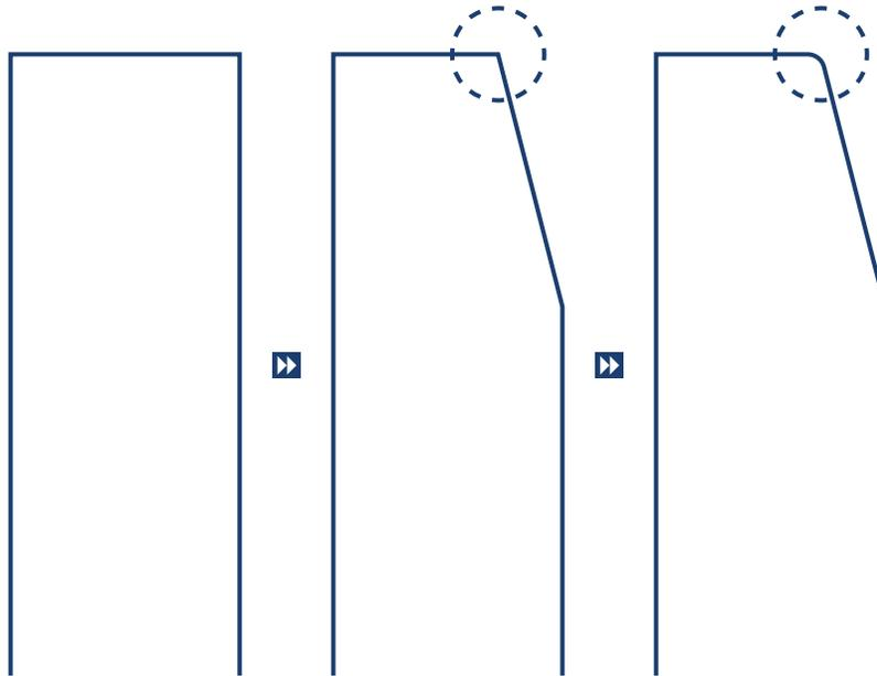
The bedknives on the Mobius are designed as semi-consumables - once the edge begins to 'roll', it's time to swap out that bed knife for a new one. To determine if your bed knife edge has rolled, run the surface of your fingernail at a 45° angle across the blade edge. If the blade edge scrapes the fingernail surface, the edge is still good. If there is no scraping of the fingernail surface, the edge has rolled and the bed knife should be replaced\*.
