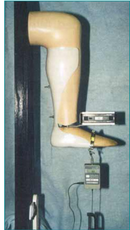
Figure 1: The model, with a single-axis hinge at the malleolar level, permits free movement from 20° of plantarflexion to 20° of dorsiflexion and is anchored rigidly to a vertical stand. Test orthoses were attached rigidly to the calf segment; static dorsiflexion resistance was measured at the metatarsal heads, to simulate the clinical effect of walking with an AFO intended to compensate for dorsiflexion weakness. A digital goniometer measured the deflection angle, and a digital tensiometer recorded the static force applied at the metatarsal head region.
