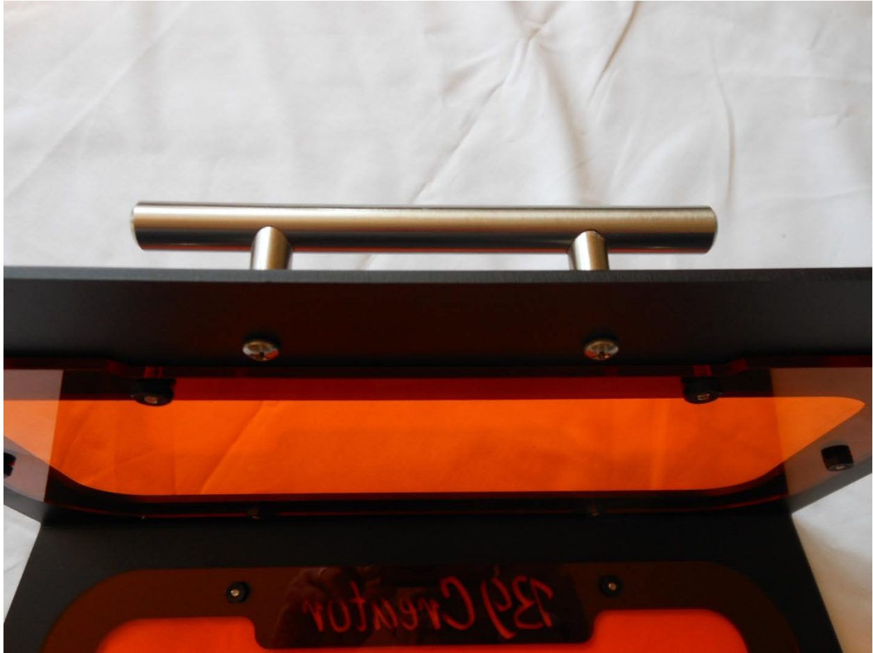
Handle secured with screws.
