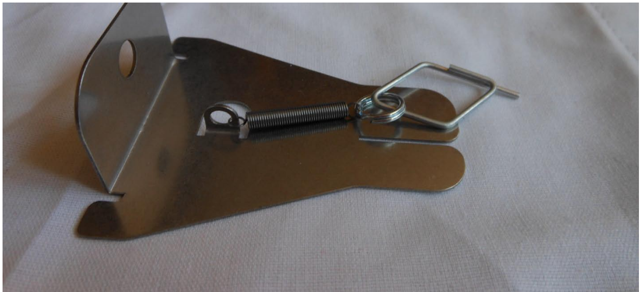
Back bracket spring assembly finished.
