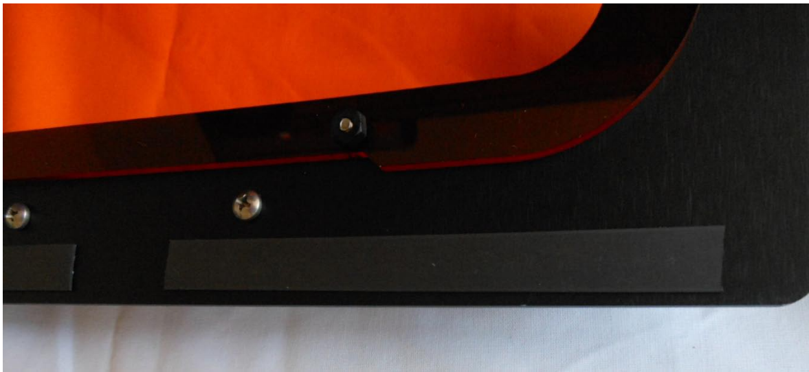
Top magnetic strips now adhered to hatch.
