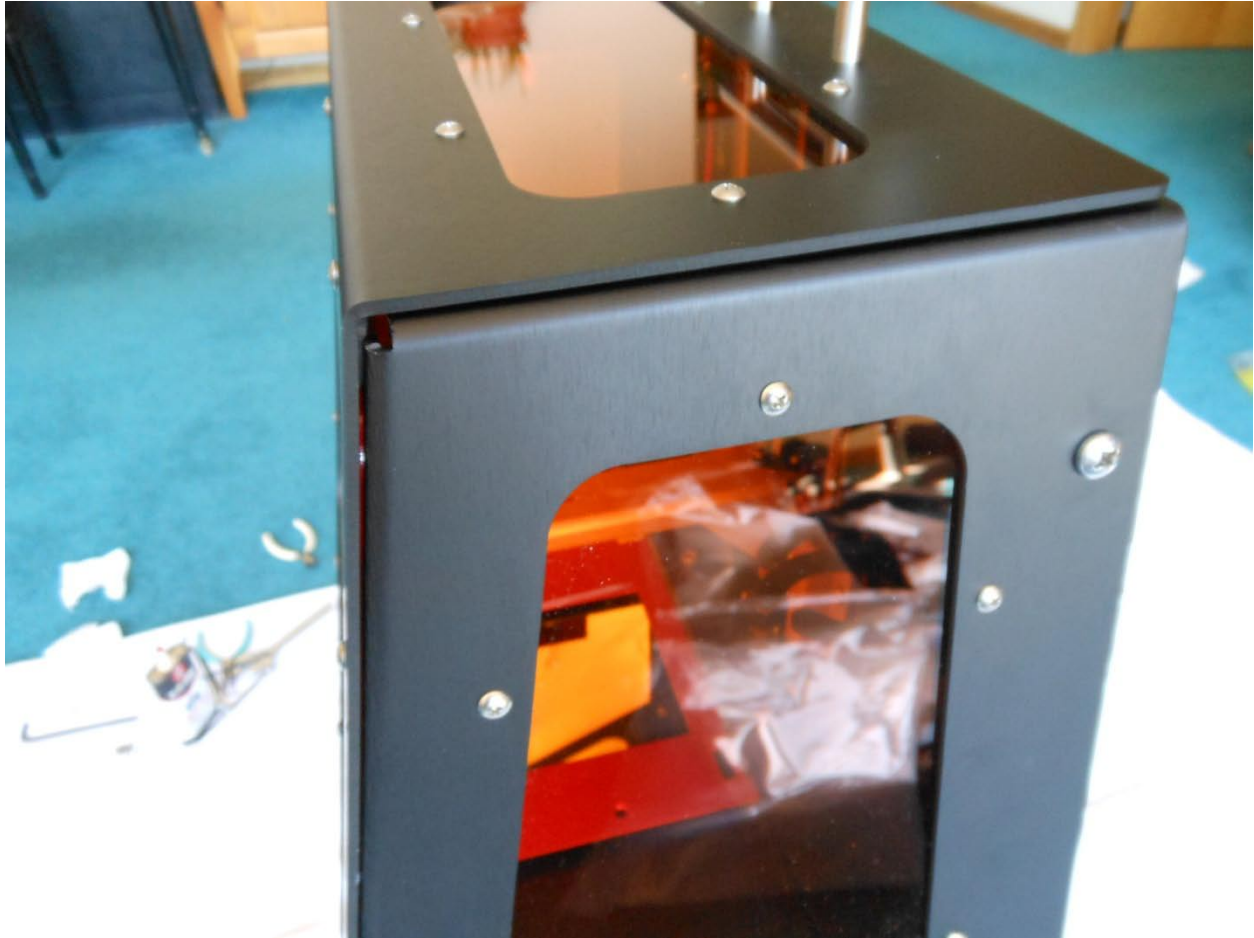
Hatch in closed position with cushions and magnetic strips.
