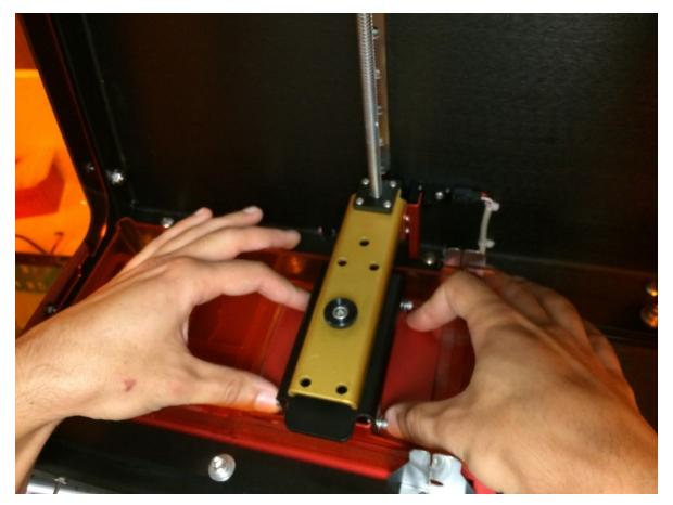
• Step 5: Ensure the bottom of the Build Table is sitting flush on the PDMS. Tighten all four build plate adjustment screws.
