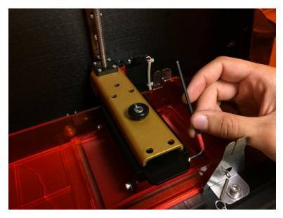
Check again if the build table is flush. If it is not, loosen the 4 screws once more, apply pressure to it and repeat this step.
