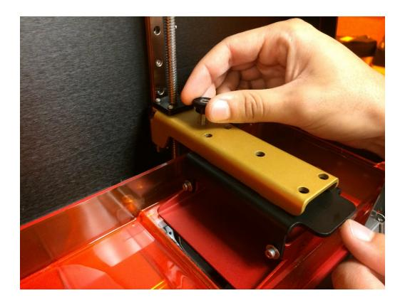
Step 7: Click here to command the printer to raise the arm out of the way.
