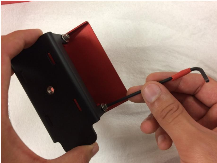
Do not remove the screws completely. They should be loose enough to allow the red build table attachment to slide up and down freely within the black, metal housing. Reattach the Build Table to the gold arm using the thumb screw. Once attached, verify that the red Build Plate is fully extended in the black housing, and the thumb screw is firmly tightened as shown in the picture below:
