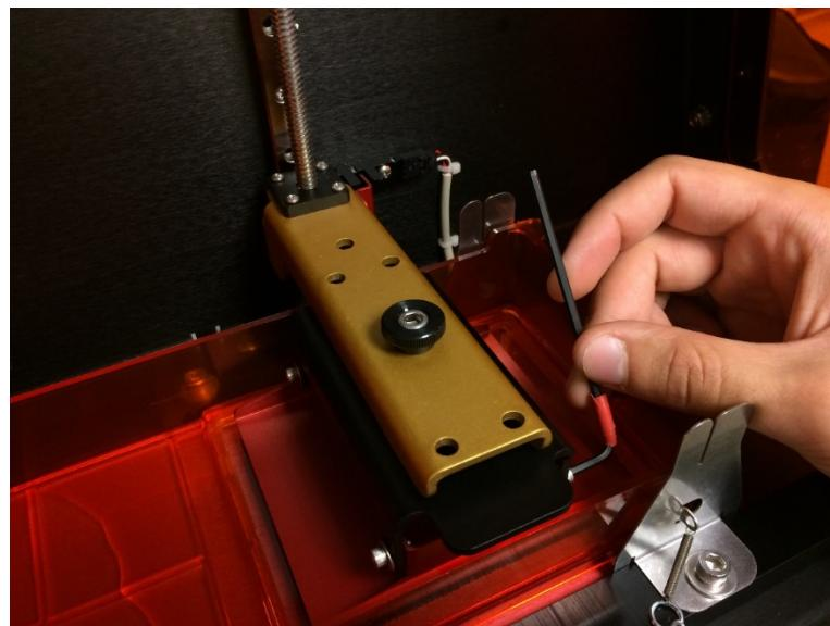
Check again if the build table is flush. If it is not, loosen the 4 screws once more, apply pressure to it and repeat this step.
