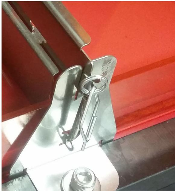
**NOTE: The springs must be attached on BOTH sides of the sweeper!**
