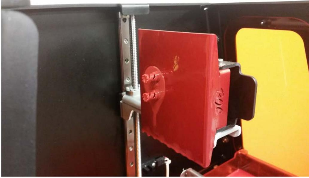
This will allow the plate to fully drain while you get ready for cleaning.
