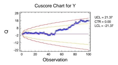
In this chart, the points plotted are the scores  $Q_j$ , calculated based on the null and discrepancy models specified on the *Analysis Options* dialog box. The centerline is drawn at 0, with control limits at
