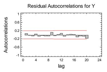
The autocorrelation measures the relationship between residuals at a specified separation in time, called the "lag". If the selected ARIMA model fits the data well, the residuals should be random and all the bars should remain within the indicated probability limits. Any bars extending beyond the limits indicate statistically significant autocorrelation between residuals separated by the indicated number of periods.
