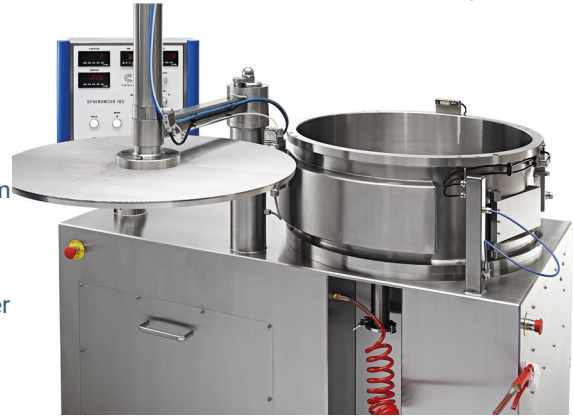
Production spheronizer disc removal system
