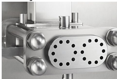
Axial configuration with 8 mm die holes
