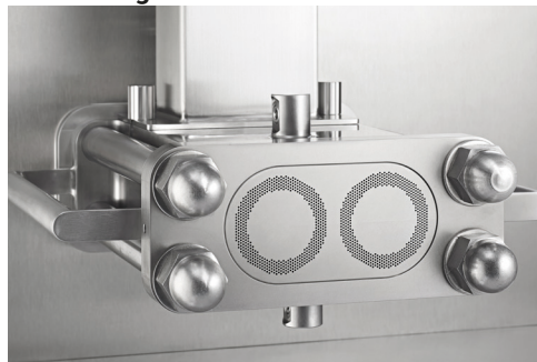
Axial configuration with 1 mm die holes
