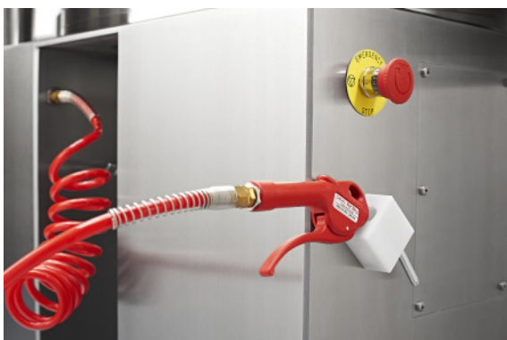
"Clean without stopping" spheronizer air blast system
