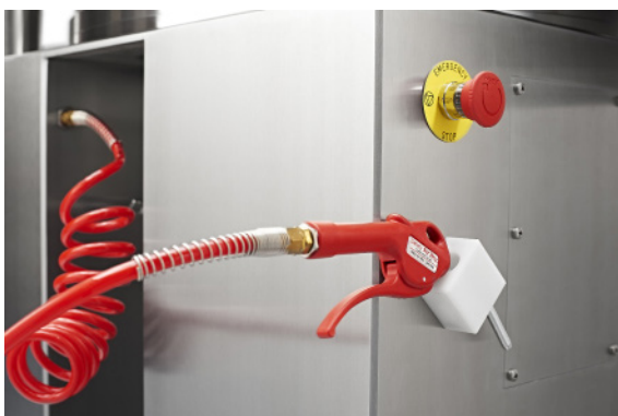
"Clean without stopping" spheronizer air blast system
