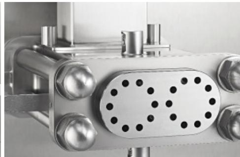
"Caleva Cone" configuration with 1 mm die holes
