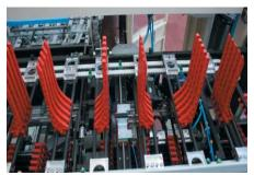
Automatic adjustment of the overhead flights. An easy and efficient system of automatic overhead flights positioning allows a quick adjustment through the operator panel.
