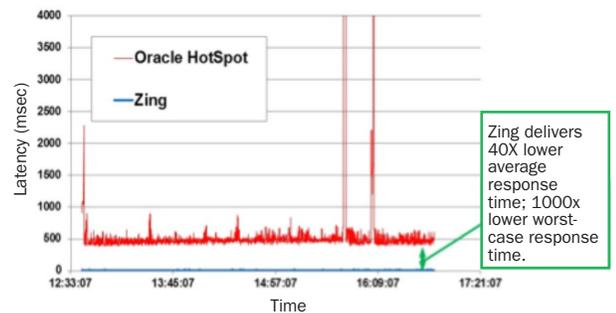
As an example of the dramatic capabilities of Zing, consider the real-world results shown in the picture above. Zing delivered an average response time 40X lower than a tuned Oracle JVM, and a 1000X reduction in worst-case response time. Same application, unchanged code – different JVMs.
