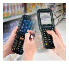
Despite the ability to operate more like their consumer grade cousins, these devices still possess many of the enterprise class features that retailers have come to depend on from their mobile computing technology including; high definition toughened glass touchscreens, 2D imaging capability, rugged drop specifications, extended battery life and more. By incorporating these enterprise features you can ensure that your mobile technology is not only fit for purpose but that it is multipurpose.
