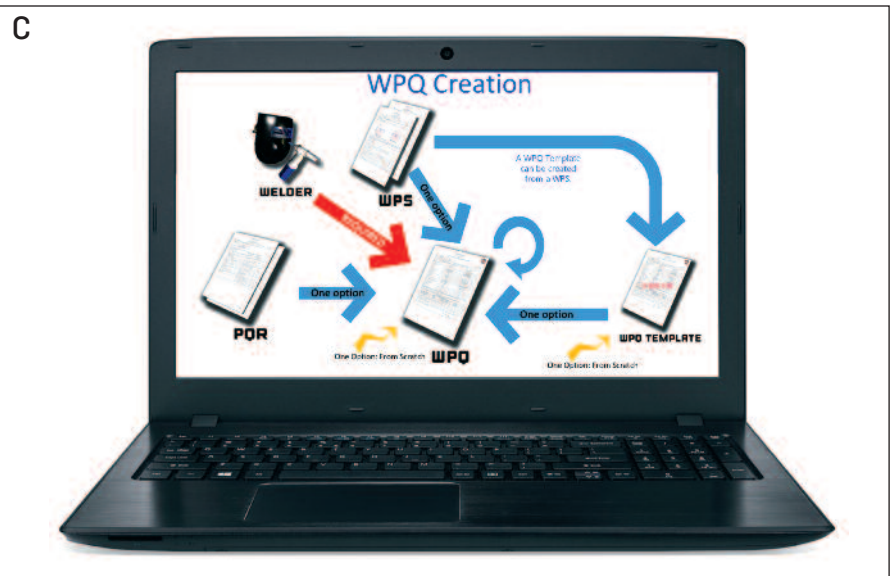
Fig. 2 — Document flows detail the creation of a PQR (labeled A), WPS (labeled B), and WPQ (labeled C).
