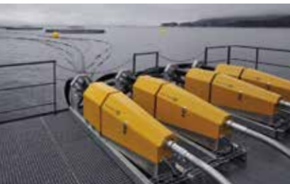
A unique feeding system All Wavemaster feed barges have built-in Akvasmart CCS Feed Systems, and the largest models are available with up to 12 parallel feed lines.
