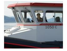
The Polarcirkel 1050 models have got new spacious cabins with entrance aft and emergency exit at the front. Both pilot and co-pilot have sliding windows.
