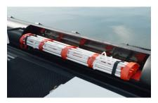
A Dacon resque net can be integrated in the pontoon. A useful and handy tool if there's an accident.
