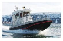
Polarcirkel Workboats are offered in three versions with inboard engines from 130hp to 435hp and lengths of 785, 845 and 910 cm.
