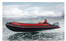
The 785 and 845 models are offered with new hull design, which gives better lift, and forces the spray out to the sides.
