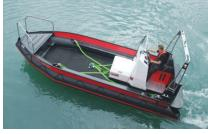
Open Workboats are also available with inboard diesel engines from 130-300Hp. The inboard series ranges from 6,60 to 8,45 meters.
