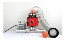
Cleaner pipes will also improve the profit. The Cleaning Sponge will be transported through the system by using pressured air.
