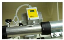
Combined with an Air Control System a reduction of transport air speed will provide significant reduction in feed dust and pellet breakage.
