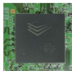
The DR Processor reduces uneven coloring, allowing documents to be scanned as images that are more suitable for OCR (Optical Character Recognition).
