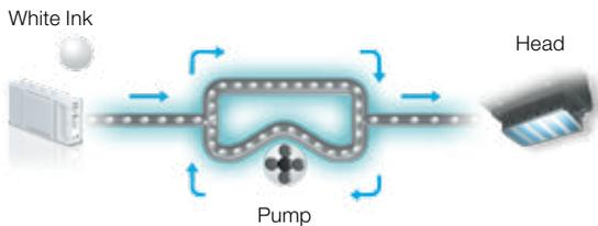
The pump circulates the white ink inside the system to prevent clogging.
