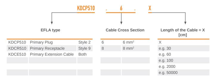
In KDCP510 and KDCR510 the other end of the cable is free. The length of the cable is given in centimeters as a suffix in the article number. For example, KDCP510.6.60 is a Style 2 Plug Connector lead with a 6 mm2 and 60 cm long cable.
