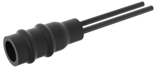
KD503 connectors have been industry requirement for over 30 years. They are designed for a fast-and-easy watertight connection between the secondary cable and the series isolating transformer. This connector is silicon and used with two single core wires. Connector is fast to install, approx. 1min. KD 503 connectors are FAA certified.
