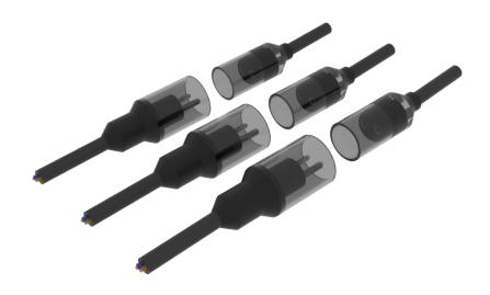
**KDC6** prefabricated extension cords meet the frangibility standards. They are equiped with a special break-away connector which is secured by an additional sleeve. If an airplane crashes with the approach light mast, connector opens safely from specific points, prevents cable rupture, and minimizes the risk of any additional hazards, like ignition of kerosin. Break-away extension cords are fully compliant with **ICAO Aerodrome Design Manual Part 6, Frangibility requirements**.
