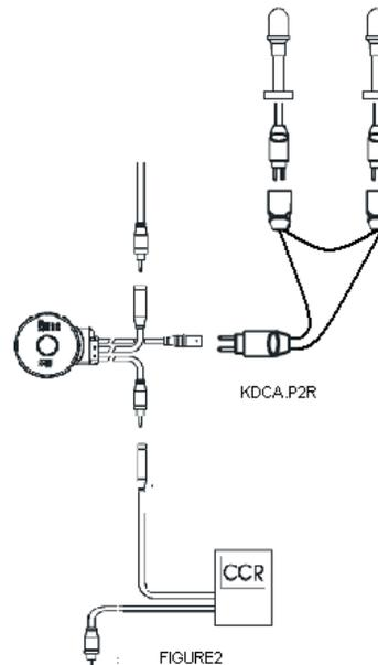
KDCA.2PR connection can be used when there is a need for a bigger power than one transformer can supply.
