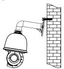
(5) Connect the cables and then hang the bracket on the wall .
