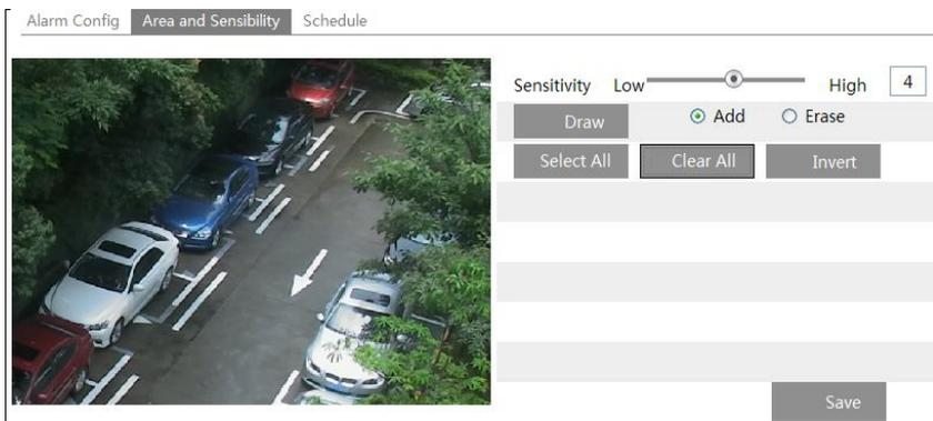
Move the “Sensitivity” scroll bar to set up the motion track sensitivity.
