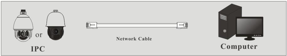
① Set the IP address of the PC and make sure the network segment should be as the same as the default settings of the IP camera. Open the network and share center. Click “Local Area Connection” to pop up the following window.
