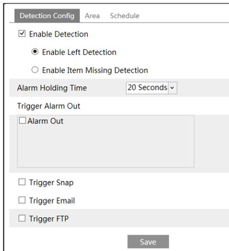
1. Enable object removal detection and then select the detection type.
