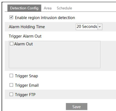
1. Enable region intrusion detection alarm and set the alarm holding time.
