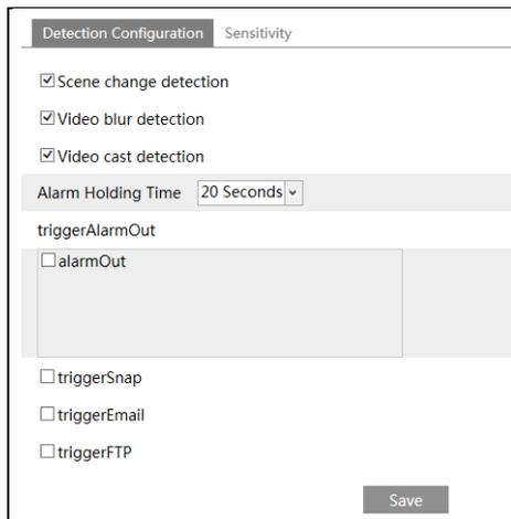
1. Enable the relevant detection as required.
