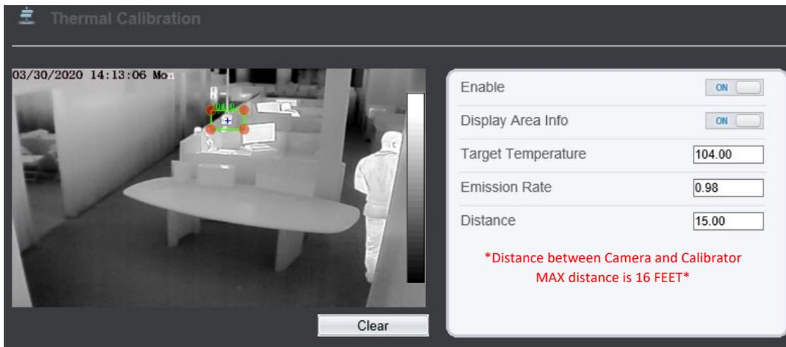
4.1 Install the blackbody properly where the camera can see it (**within the thermal image**). The blackbody needs to be powered on for at least 20 mins to reach to a stable temperature.
