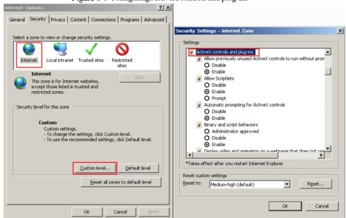
Figure 8-9 Configuring ActiveX controls and plug-ins
