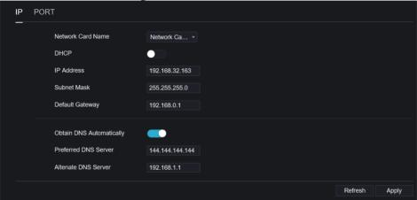
Step 2 Choose network card from the drop-down list. Network card I is LAN1, network card II is LAN2, as shown in Figure 9-24.
