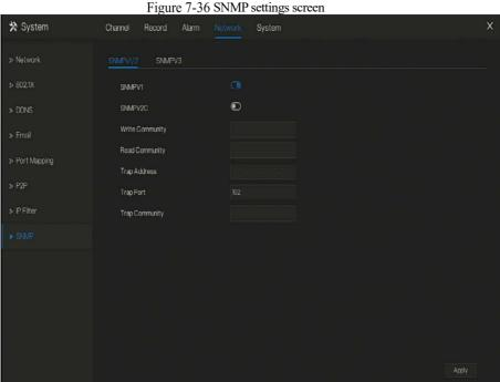
Step 2 Click next to SNMPV 1 to enable the function. The interface is shown as Figure
