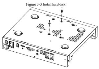
Step 5 Insert the hard disk data cable and power cable, then put on the upper cover and fasten the fixing screws.
