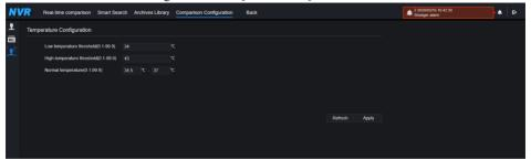
At temperature comparison interface, user can set low temperature threshold, high temperature threshold, normal temperature, as shown in Figure 8-38.
