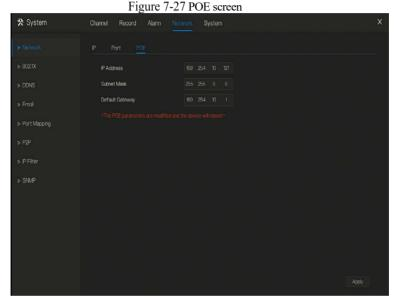
Step 2 The NVR will deploy IP addresses to the cameras which connect POE immediately.
