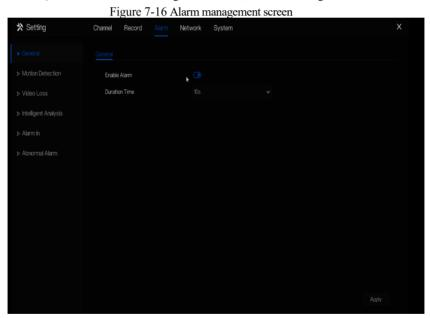
Step 2 Enable the Enable alarm button.
