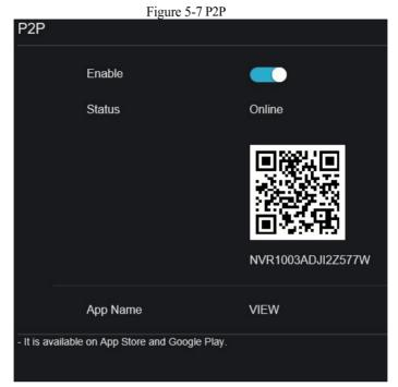
Step 8 Enable the P2P, user can use mobile devices to manage the NVR by scanning the P2P ID, if the mobile phone has loaded the InVid LIVE app(search the APP at App Store or Google Play).
