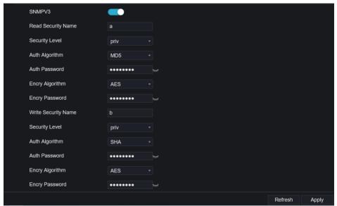
Step 2 Input the information of SNMP (simple network management protocol) . there three types of that function. User can apply that if need.
