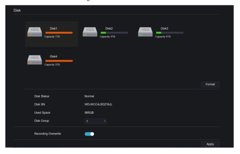
Step 2 You can view the information like capacity, disk status, disk SN code and used space.
