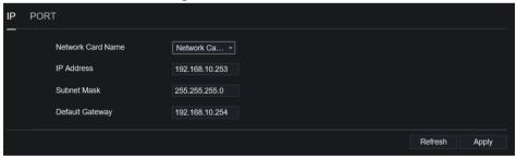
Step 3 Click next to **IP** to enable or disable the function of automatically getting an **IP** address. The function is enabled by default.
