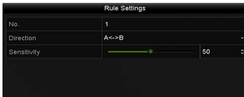
Figure 9. 4 Set Line Crossing Detection Rules
