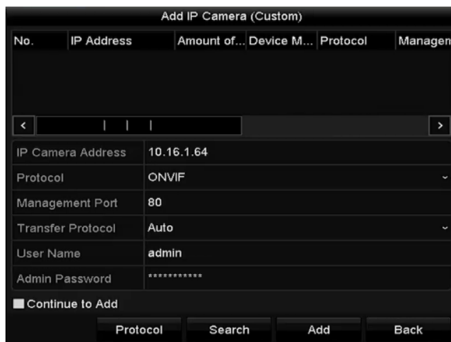
Figure 2. 22 Custom Adding IP Camera Interface
