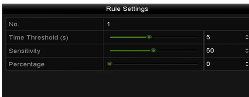
Figure 9. 6 Set Intrusion Crossing Detection Rules
