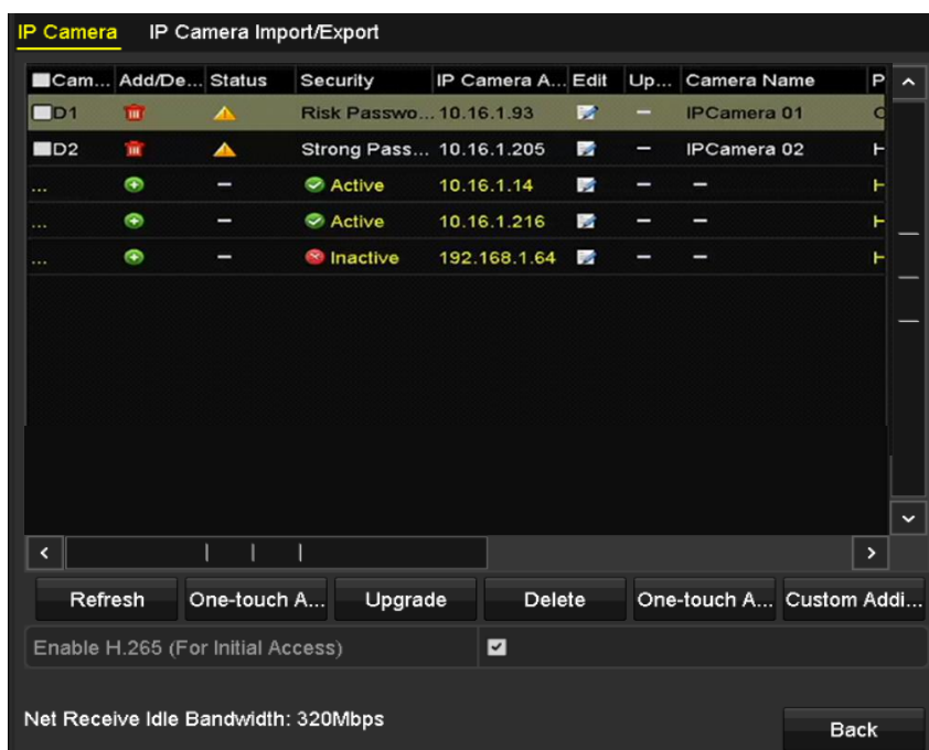
Figure 2. 20 Adding IP Camera Interface
