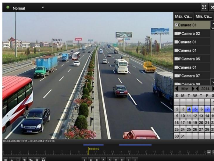
Figure 6. 8 Interface of Playback by Time
