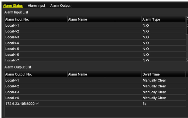
Figure 8. 4 Alarm Status Interface of System Configuration
