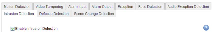
Figure 6. 6 Setting Intrusion Detection on IP Camera
