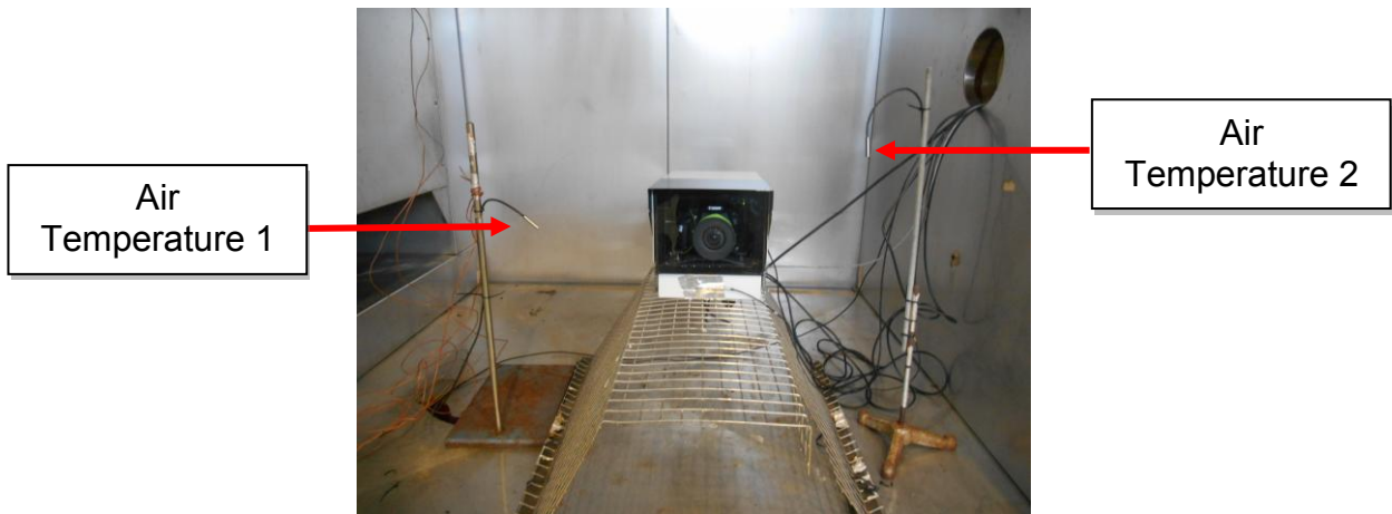
TEMPERATURE TEST – CHAMBER CONFIGURATION
