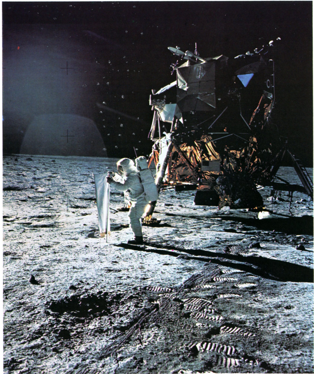
Aldrin deploys instruments to collect particles of "solar wind."
