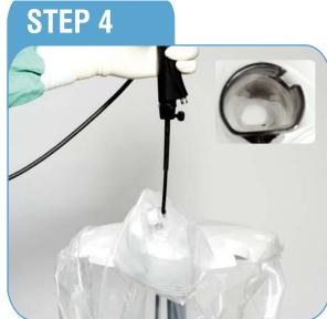
Gently insert scope into EndoSheath protective barrier with the endoscope label facing forward and the flat edge of the insertion tube against the flat edge of the EndoSheath protective barrier connector opening.
