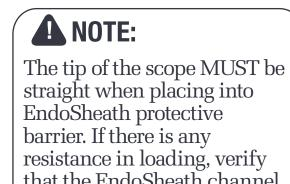
resistance in loading, verify that the EndoSheath channel is properly aligned. If the channel is misaligned/twisted, straighten the channel before continuing scope insertion.
