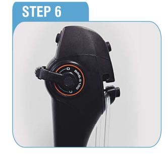
When using the BVX-1.5 or BVX 2.1 EndoSheath protective barrier, insert suction tube through the suction pinch valve.
