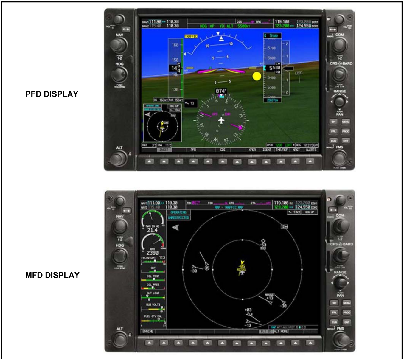
FIGURE SB-321-7 - ADS-B "OUT" and "IN" DISPLAYED ON G1000
