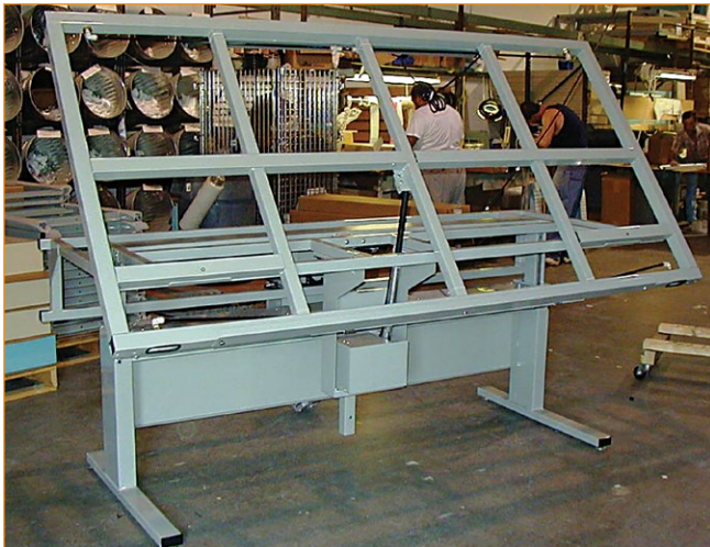
Workers for a large jet manufacturer use 32 custom Model WHJ9648-80-EX electric workbenches to assemble the aircraft's 32-foot long wire harnesses. Photo courtesy Proline
