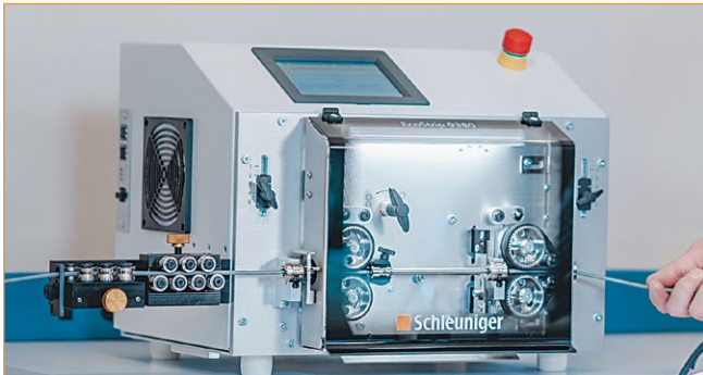
The Northcomm Technologies Group processes five types of cable on the Schleuniger EcoStrip 9380 machine. Photo courtesy Schleuniger Inc.
