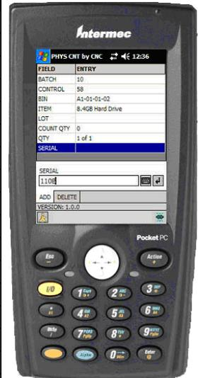
When a Purchase Order Receipt is completed on the handheld, the user can optionally be prompted to print bar coded labels for that item to a desktop or portable RF belt printer.
