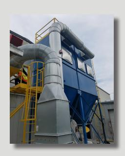
**A.C.T. Dust Collectors** TLM Modular Baghouse is designed to meet the unique requirements of each application.
