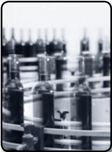
Guide rail used in a filling application
